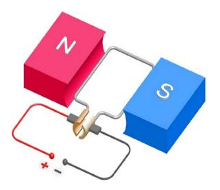
a) Label the split ring commutator and carbon brushes and explain the function of these two parts.
